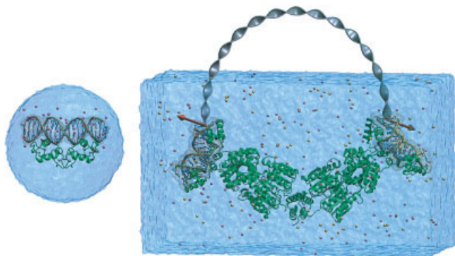
Figure 1. Growth in practical simulation size illustrated by comparison of estrogen receptor DNA-binding domain simulation of ref. 5, left, 36,000 atoms simulated over 100 ps, published in 1997, with multiscale LacI–DNA complex simulation of ref. 6, right, 314,000 atoms simulated over 10 ns, published in 2005 and described in the exemplary applications section. [Color figure can be viewed in the online issue, which is available at www.interscience.wiley.com .]
